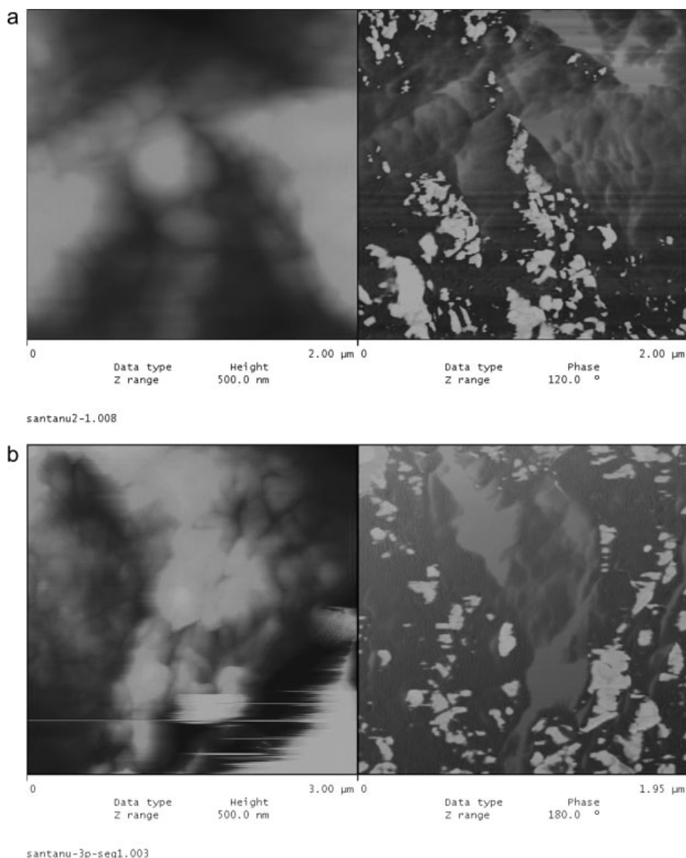
Figure 3 Height and phase AFM images of (a) ELS 6/4/3-3 and (b) ELS 6/4/3-3/Si-69. [Color figure can be viewed in the online issue, which is available at www.interscience.wiley.com .]
